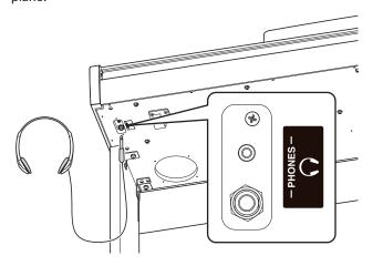
Up to two pairs of headphones can be connected and used simultaneously. When a pair of headphones is connected, sound will not be produced by the speakers.
